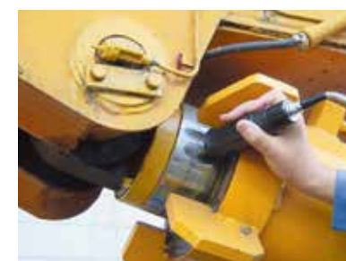
● Diagnosing wear and tear using hardness measurements
