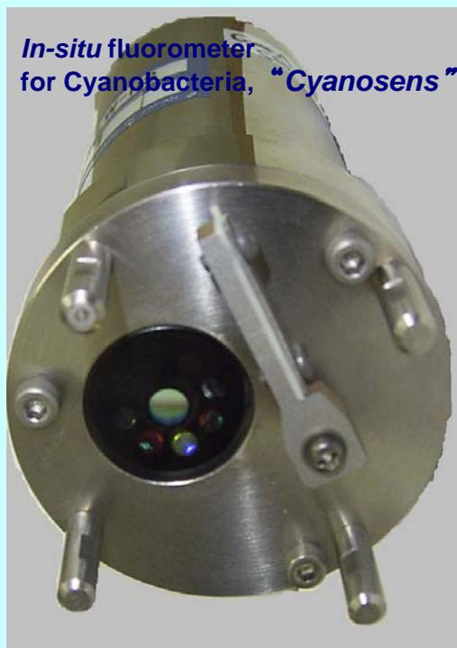
*In-situ* fluorometer for Cyanobacteria, “Cyanosens”
