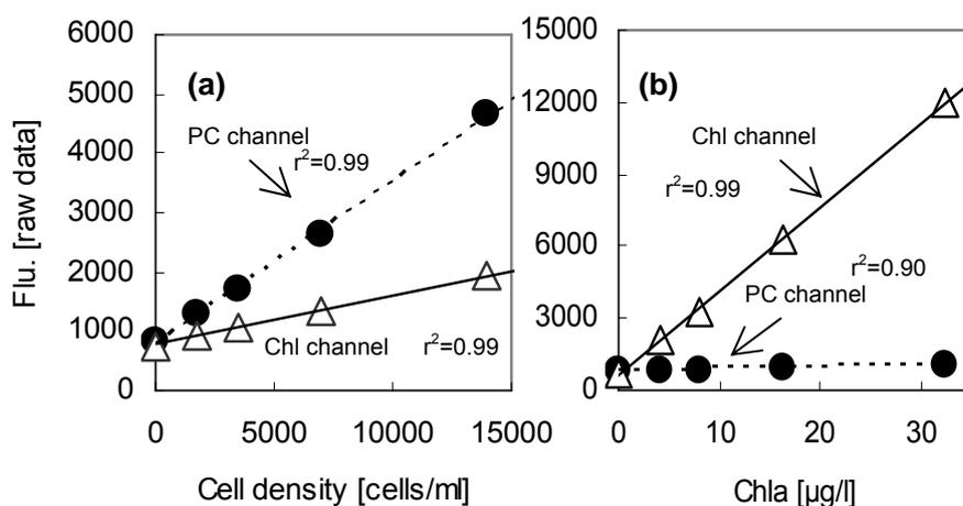
**Fig.4** Relationships between (a) PC fluorescent intensity and cells density of cyanobacteria, *A. affinis*, (b) Chla fluorescent intensity and Chla concentration of diatom, *S. costatum*. These tests were done using culture collection.
