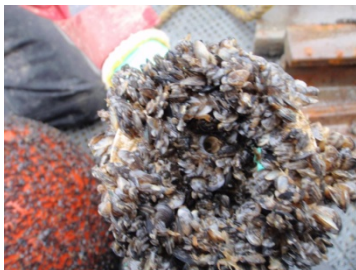
Bio-fouling covers the ACTW instrument but the conductivity electrode is clean by the anti-fouling wiper.
