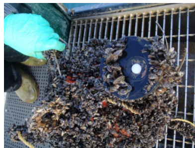
Wiping performance of ACLW2 chlorophyll and turbidity sensors and ALW PAR sensor.
