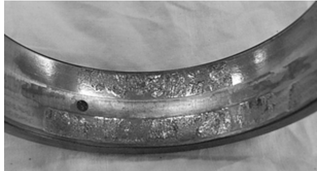
Fig.2 Failure on the outer race of the bearing of the step chain sprocket ( E_{area}=1\ 018[\text{dB}^2] )
