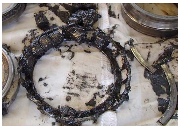
Fig.5 Damaged bearing at the step chain sprocket due to severe unlubrication ( E_{area}=7[\text{dB}^2] )
