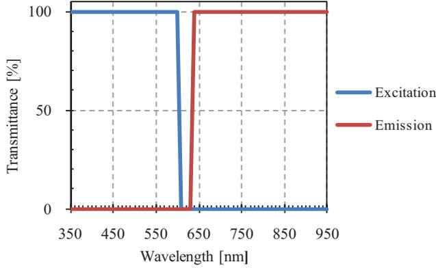
Figure 2. Characteristics of the optical filters.
