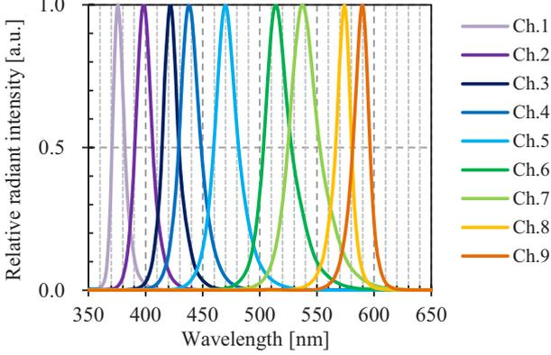
Figure 1. Spectral distributions of the nine LEDs.
