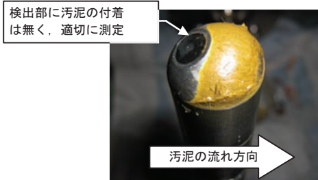
Fig.10: Situation of The Adhesion of Sludge to The Detector (Low Flow Rate, 0.2m/s)
