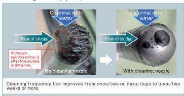
By using a cleaning nozzle, sludge adhesion is prevented even with highly viscous concentrated sludge.
