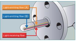
The detector section irradiates two types of near infrared rays (A and B) from the end of the emitting optical fibers, receives the scattered light reflected from the sludge in the receiving optical fiber and converts it to an electrical signal.
