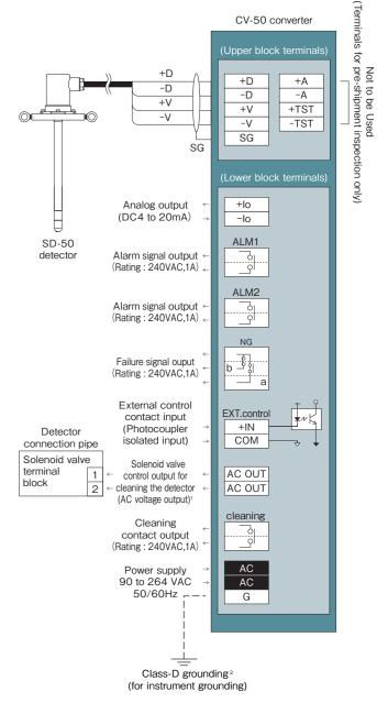
1:The AC voltage output to the solenoid valve control output for cleaning the detector (AC OUT) is the same as the power supply voltage (90 to 264VAC 50/60Hz) to the converter.
