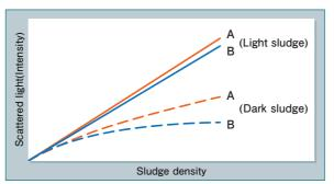
The scattered light intensity of the received light is determined by the density and color of the sludge for each wavelength of the light. SD-50 reduces the influence of the sludge color through automatic correction using the difference of the correlation characteristic.
