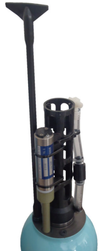
Float and CTD sensors not manufactured by JFE Advantech.
