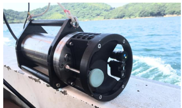
Fig. 4 Underwater spectrophotometer developed by JFE Advantech Co., Ltd. The instrument carries additional temperature, conductivity, chlorophyll-a fluorescence and fast optical dissolved oxygen sensors.
