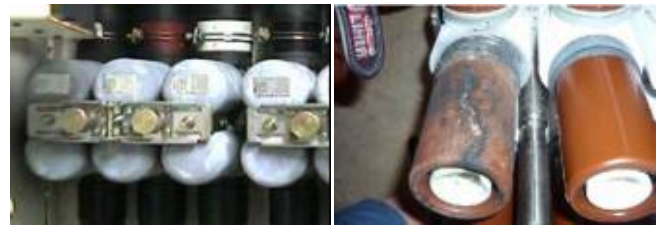
図4 AE検知されたMDS(左)と電極内部状況(右) Fig. 4. Damaged MDS detected by means of AE (left) and its failure of inside electrode (right).
